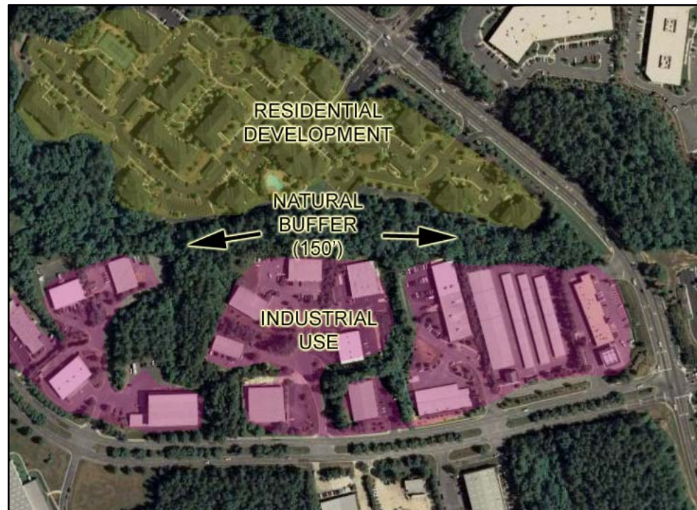
Fig. 2-6: Example of Buffer between Incompatible Uses
